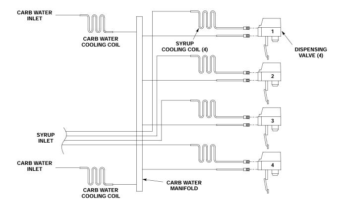
FIGURE 4. PLUMBING DIAGRAM (FOUR-FLAVOR UNIT REQUIRING REMOTE CARBONATOR)
